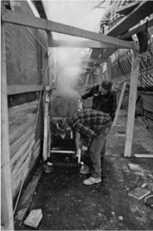
The steam box in use. Wood-fired steam created to heat planks of oak for bending to create shape of hull. This was the last boat to be built on the coast using this old method of wooden boat building.
